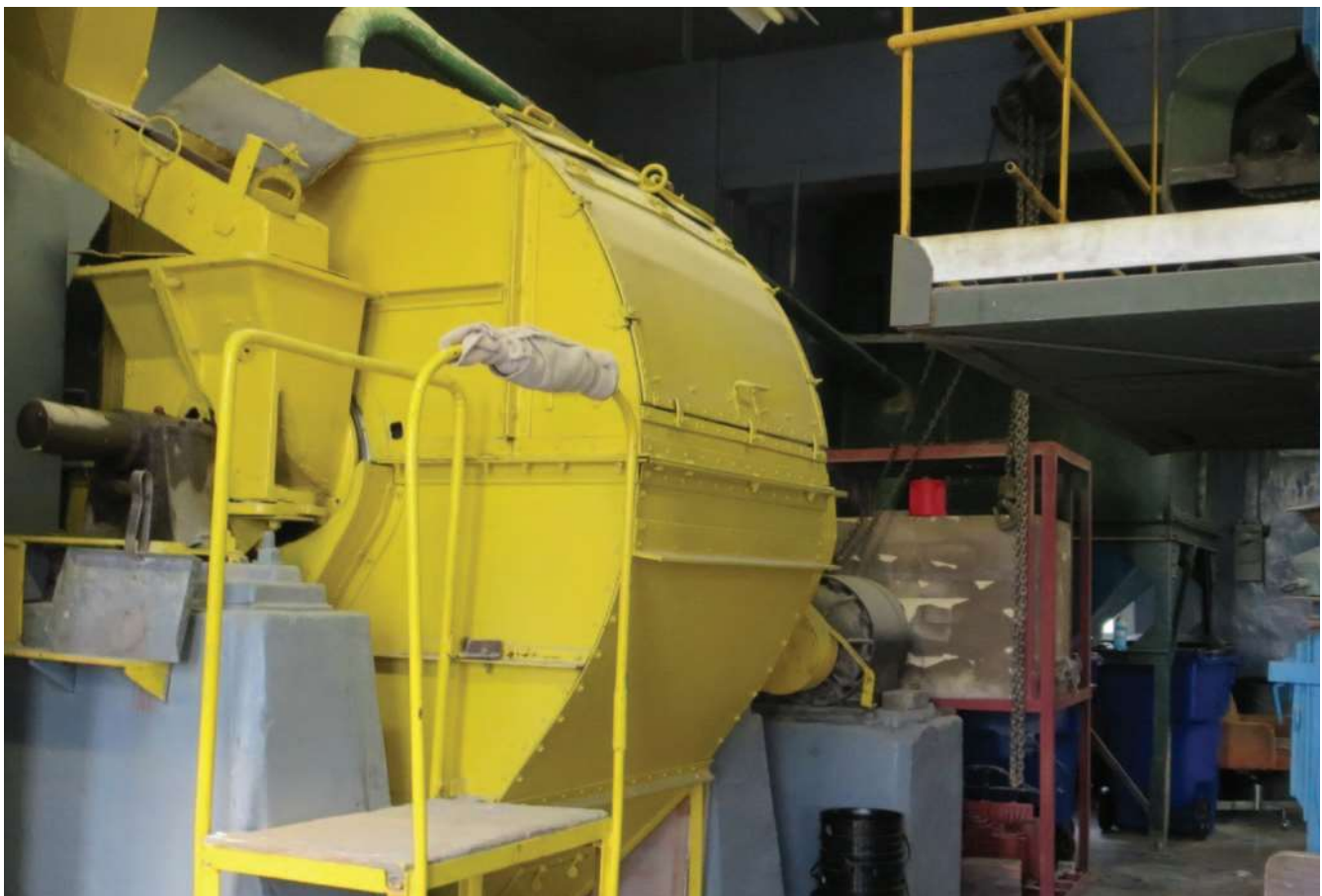
Clockwise from top: TTL’s cone crusher; the TTL was built in the 1940s by the provincial government to serve the needs of miners in Cobalt, Ont.; scoop tram at the Castle mine adit entrance; TTL’s ball mill.
