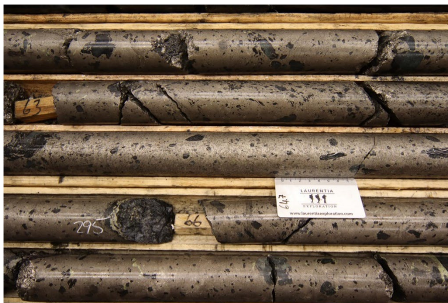
Zoomed in core photo of GRL-22-60 showing the massive sulphides (News Release February 16, 2023)
