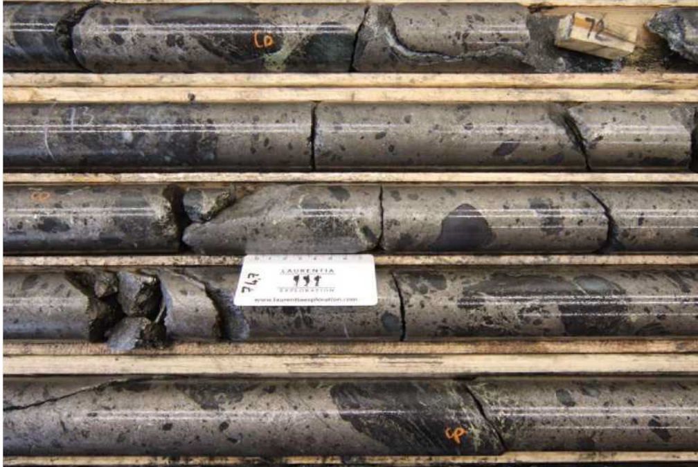
Figure 8: Example of massive sulfide mineralization in wet drill core at Graal (GRL-22-61; Box 17-19: 71.70 m - 77.60 m)
