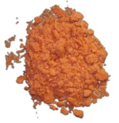
Fig. 4: Cobalt sulphate produced from Castle Mine concentrate using the re-20x process
