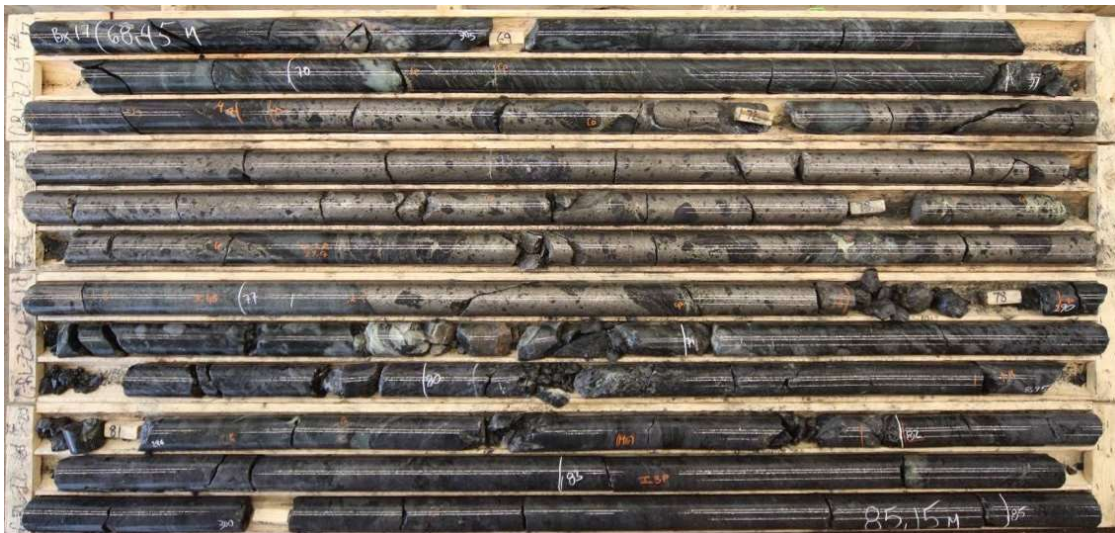
Core photo of GRL-22-61, highlighting the sulphide intersection between 62.10 to 77.80m (News Release February 16, 2023)
