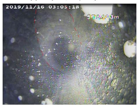
Figure 32: Vein contact with weight at 2 O'clock and contact at 11 O'oclock
