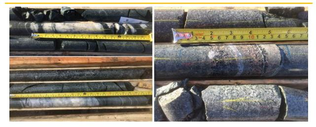
Figure 15: Drill core with veins mostly filled by quartz cements within the Nipissing diabase
