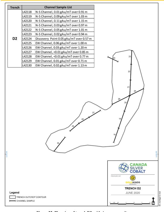
Figure 25: Plan view of trench D2, with Au assay results
