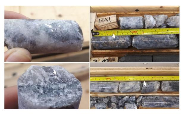
Figure 13: Underground drill core showing silver-cobalt-nickel mineralisation (white arrows)
