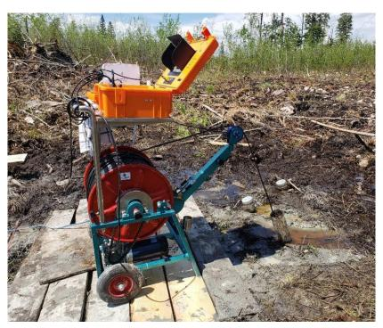
Figure 36: The camera down hole CS-20-22.
