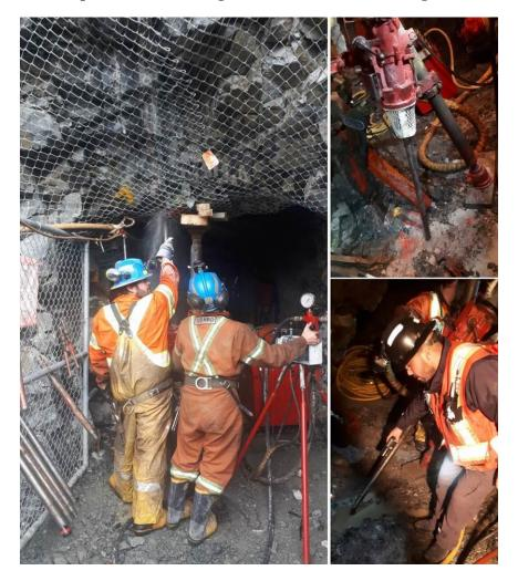
Figure 44: Underground drilling with electrical drill (drill size AQ)
