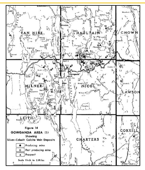
Figure 6: Gowganda Area Showing Silver-Cobalt Calcite Vein Deposits (modified after Sergiades, 1968)
