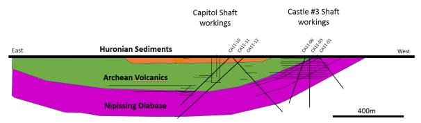
Figure 11: Schematic geological cross section lookin SW (Modified from Robinson, 2015)
