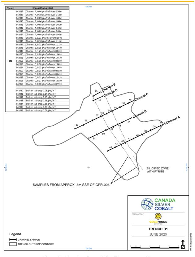
Figure 24: Plan view of trench D1, with Au assay results
