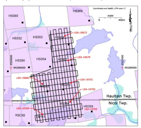
Figure 27: Location of mining leases and drone's path (Zen Geomap inc., Report - Drone Magnetometer survey)
