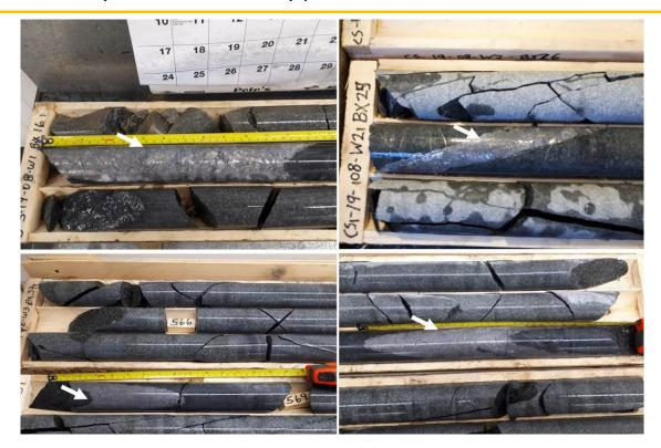
Figure 14: Massive silver-cobalt mineralisation (white arrows) intersected by the drill holes (wedges program 2019/2020)
