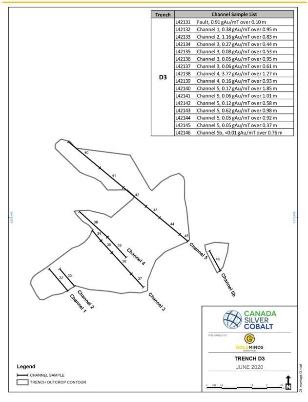
Figure 23: Plan view of trench D3, with Au assay results
