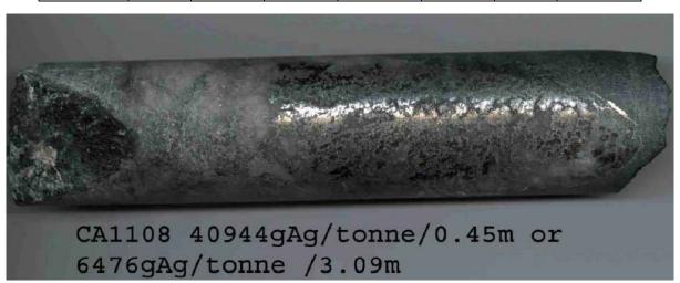
Figure 17: Massive silver mineralisation intersected at drill hole CA1108
