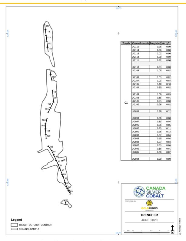
Figure 26: Plan view of trench C1, with Au assay results
