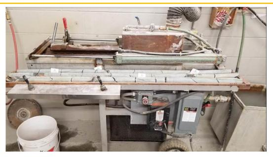
Figure 49: Electrical saw used for cutting the core samples
