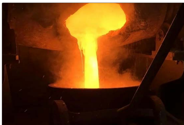
Figure 9: Silver dore pour at TTL facility
